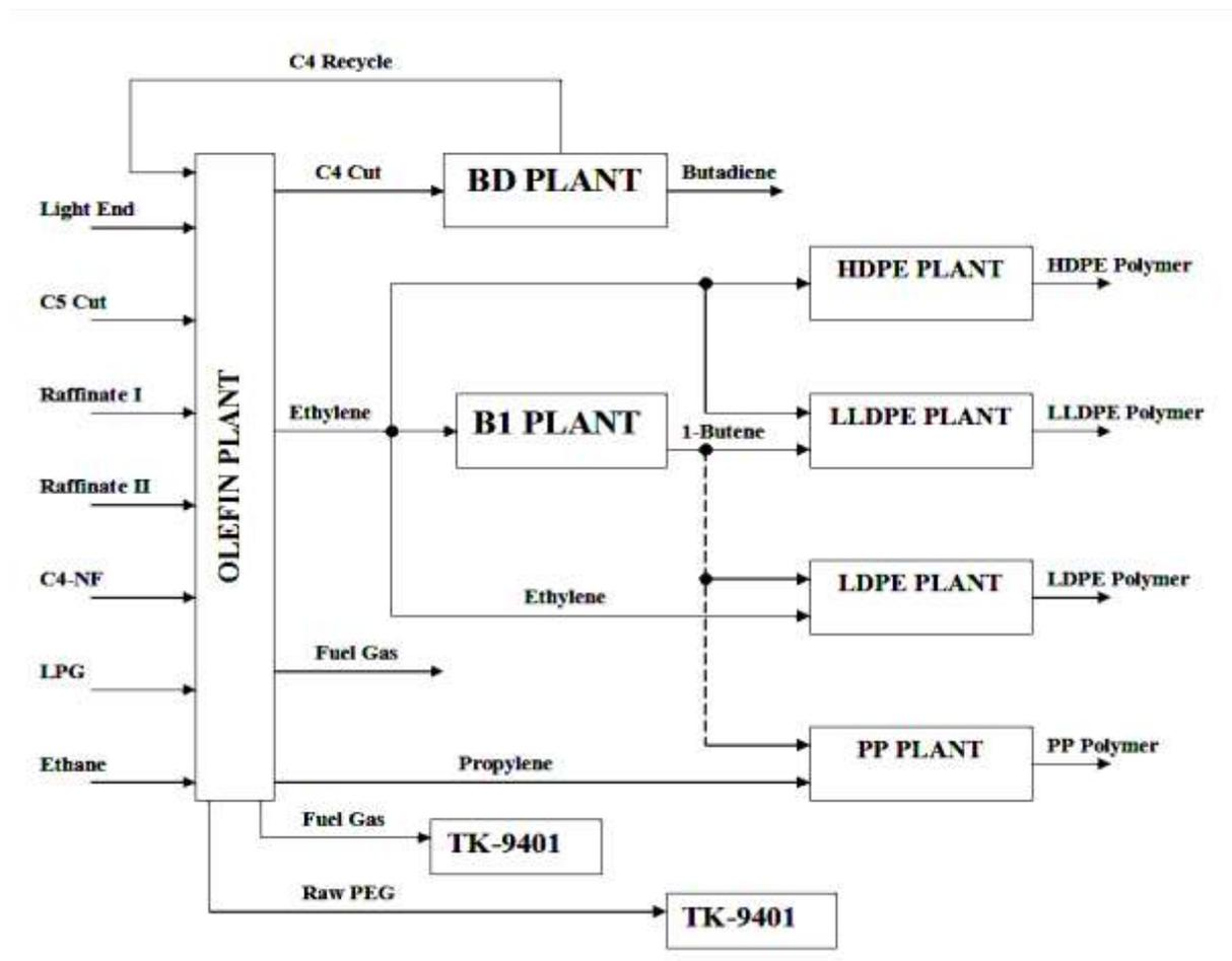
**Figure 2:** Brief process diagram of Amirkabir petrochemical complex
