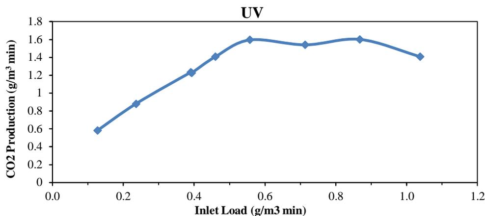
**Figure 5.** CO<sub>2</sub> production against the ethylbenzene inlet load in photocatalytic reaction
