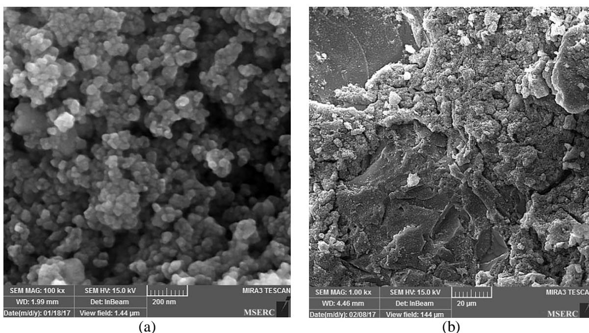
**Figure 2.** FE-SEM images of (a)  $\text{TiO}_2$  catalyst, and (b) the surface of coated glass bead
