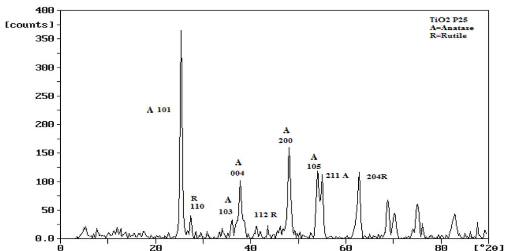
**Figure 1.** XRD pattern of Degussa P25 catalyst
