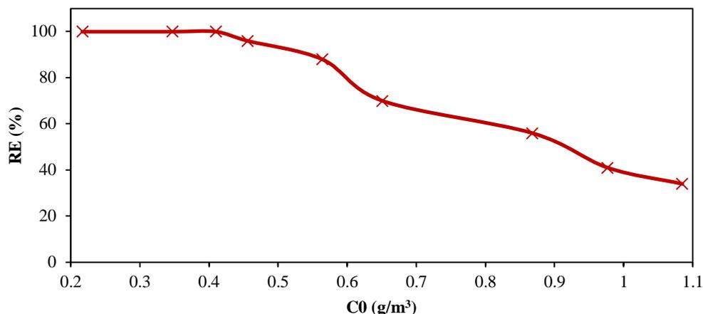
**Figure 3.** Effect of inlet concentration on removal efficiency at 1 min residence time.
