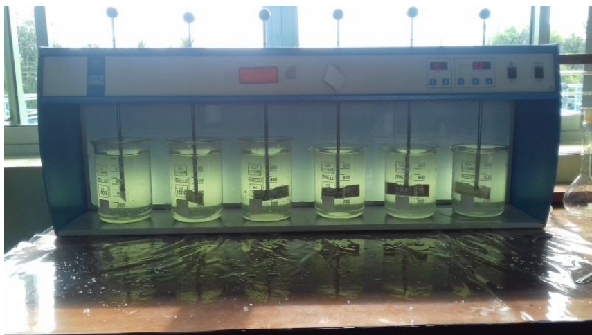
Figure 1. Removal of turbidity at different dosages of coagulants using jar test
